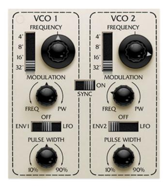
Synthesizer Expander Module includes two almost identical voltagecontrolled oscillators. The only difference are their modulation routing options.
